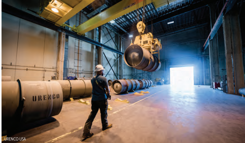
CYLINDERS OF URANIUM HEXAFLUORIDE are processed at Urenco USA's enrichment plant in Eunice, New Mexico. The sole US commercial uranium enrichment facility, it provides about one-third of the nuclear fuel used by domestic nuclear power plants.
