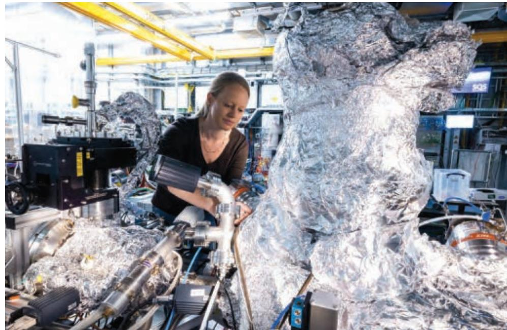
**FIGURE 1.** REBECCA BOLL works on the Small Quantum Systems instrument at the European X-Ray Free-Electron Laser. Wrapped in aluminum foil is the reaction microscope, which captures the charged fragments of molecules blown up by the powerful x-ray pulses. The foil insulates the equipment while the researchers bake out the residual gases. (Courtesy of European XFEL/Jan Hosan.)
