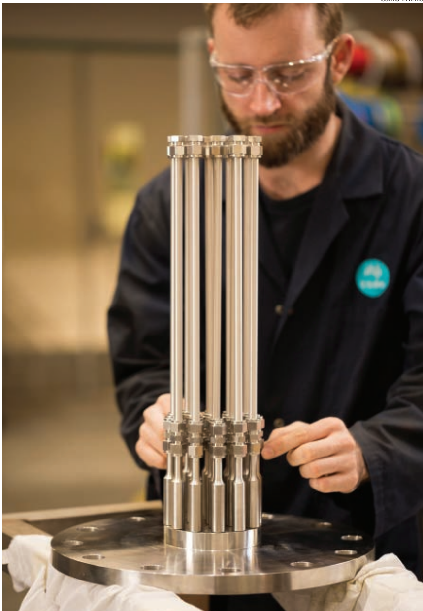
CSIRO ENERGY BUILT AND DEMONSTRATED this vanadium-based membrane system for extracting pure hydrogen from ammonia. It's currently being scaled up to produce 200 kg/day.
