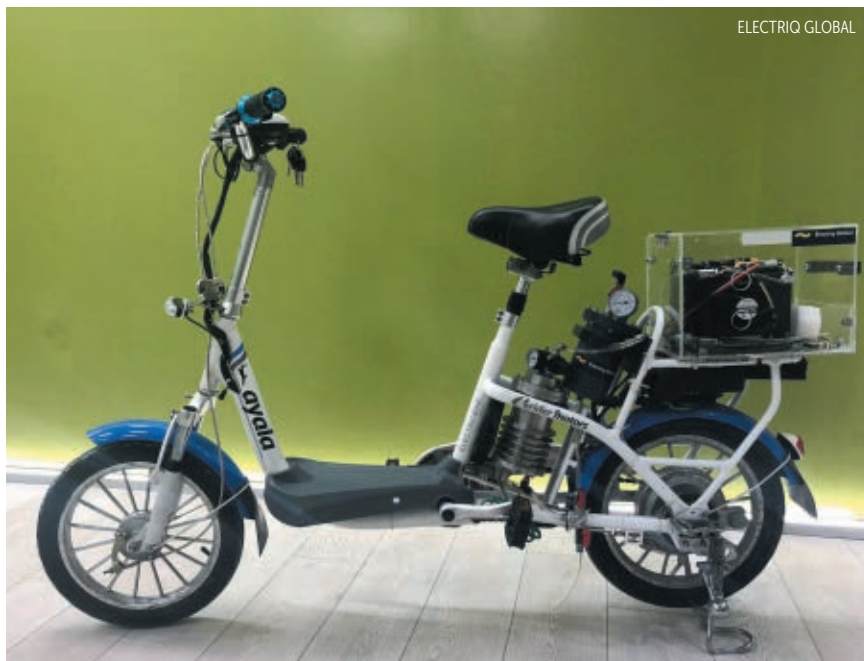
A MOTORIZED BICYCLE demonstrated the potassium borohydride system that Electriq Global is developing as a hydrogen source for fuel-cell electric vehicles.
