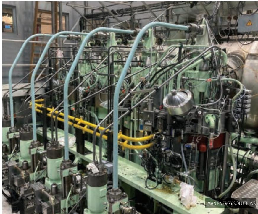
**A PROTOTYPE** ammonia-powered ship engine built by MAN Energy Solutions. The company is now building a commercial engine for a Japanese shipbuilder.
