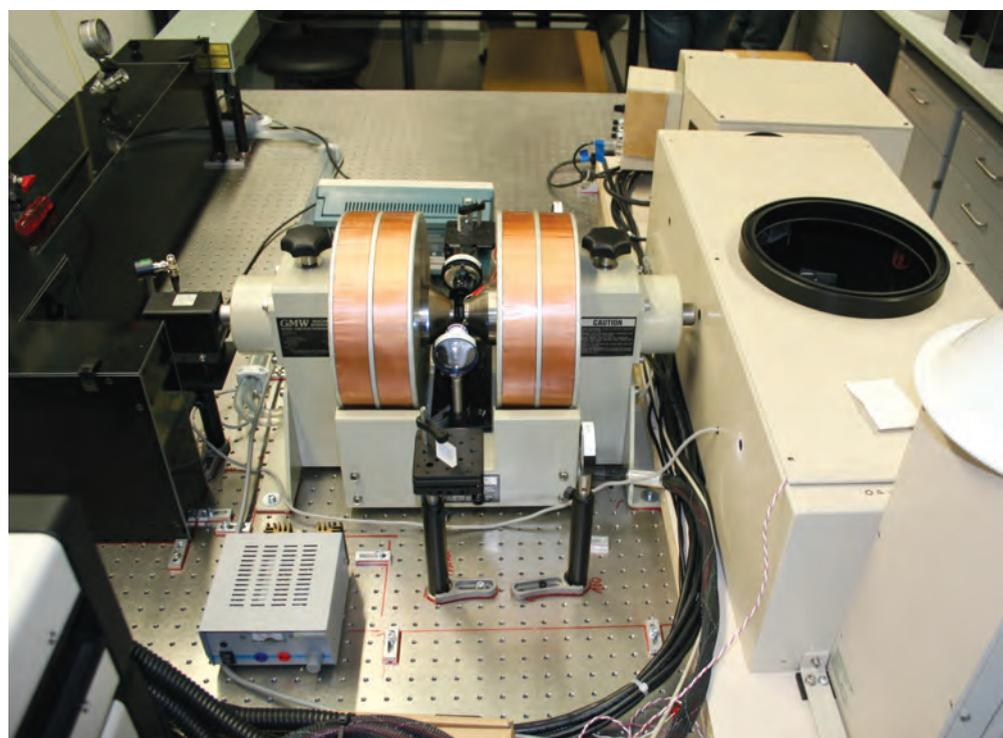
**FIGURE 1. TWO ELECTROMAGNET COILS** flank a sample chamber containing a solution of photoactive molecules. The surrounding optics direct a pair of laser pulses at the sample to manipulate the molecules' spin dynamics. (Courtesy of Michael Moos.)
