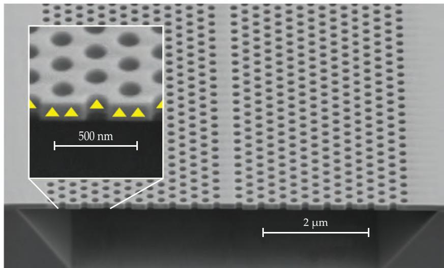
**FIGURE 4. THIS ON-CHIP WAVEGUIDE**, taken with a scanning electron microscope, consists of a hexagonal arrangement of holes etched in a gallium arsenide membrane. The row of missing holes constitutes the waveguide. The yellow triangles (inset) indicate the position of the quantum dots in the center of the membrane. (Adapted from ref. 2.)
