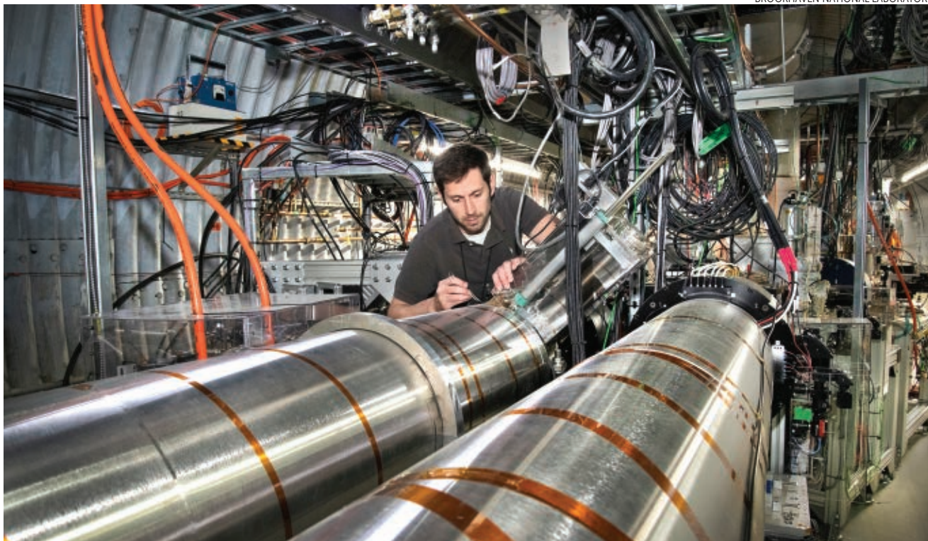
BROOKHAVEN NATIONAL LABORATORY ENGINEER MATHEW PANICCIA next to accelerator beamlines in which low-energy electrons commingle with ions to extract heat and keep the ion bunches tightly packed. The approach may be applied in high-energy hadron cooling in the electron-ion collider.
