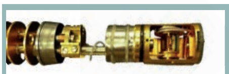
Rotating sample platform for 300 mK operation
