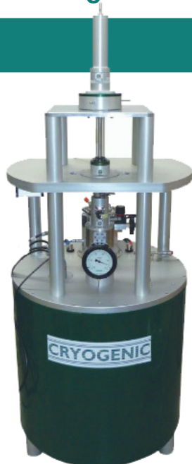
Rotating sample platform for 300 mK operation
