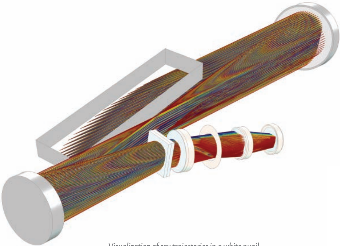
Visualization of ray trajectories in a white pupil échelle spectrograph.
