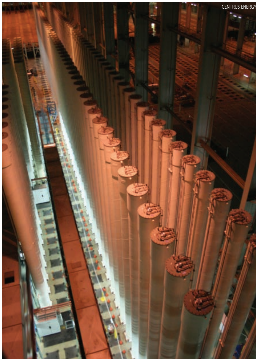
CENTRUS ENERGY IS BEING AWARDED a no-bid contract from the Department of Energy to demonstrate the production of high-assay low-enriched uranium using 12-meter-tall centrifuges, shown here.
