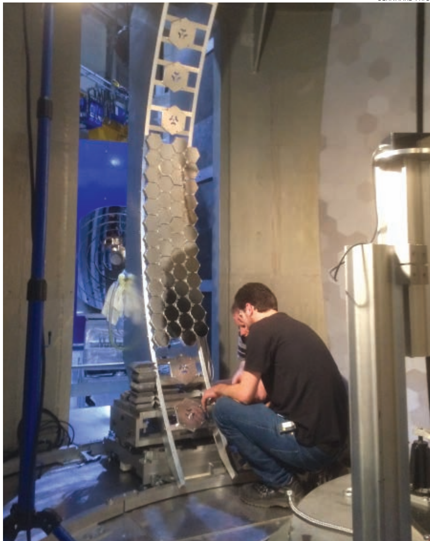
FIGURE 1. KRISTIJAN KUHLMANN (front) and Markus Appel (back, almost hidden) examine part of a gallium arsenide analyzer in a proof-of-concept neutron backscattering spectrometer. In a fully functional spectrometer, the hexagonal GaAs facets will cover about 20% of the surface area of a sphere centered on the sample (right foreground).
