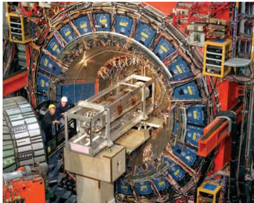
**FIGURE 1. THE COLLIDER DETECTOR** at Fermilab's now-defunct Tevatron accelerator measured the positions and momenta of electrons and muons produced in proton-antiproton collisions as they passed through 30 240 high-voltage wires. The detector provided data for the highest-precision measurement of the W-boson mass to date. (Courtesy of Reidar Hahn/Fermilab.)
