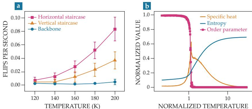
**FIGURE 2. ENTROPY-DRIVEN ORDER** in tetris ice can be studied in quantitative detail. (a) Imaging of the system over time shows that the staircase moments, where the lattice entropy is concentrated, change their magnetization much more frequently than the backbone moments, which are driven toward order. (b) A Monte Carlo simulation exhibits an order–disorder phase transition, despite the system’s residual entropy at low temperature. (Adapted from ref. 1.)
