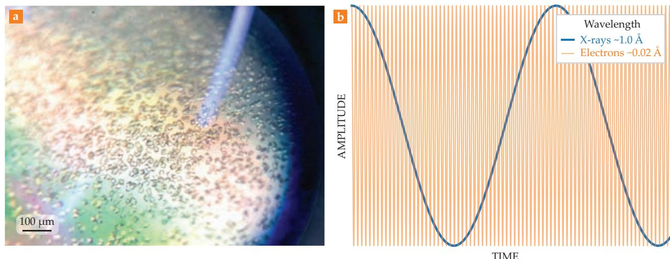
**FIGURE 1. CRYSTALS** and their diffraction. (a) Protein crystals of proteinase K, a serine protease, are seen through a light microscope. (b) The graph shows a comparison between the wavelengths of x rays (blue) and electrons (orange) typically used in diffraction experiments. With their much shorter wavelength, electrons can resolve much finer details of a biomaterial.
