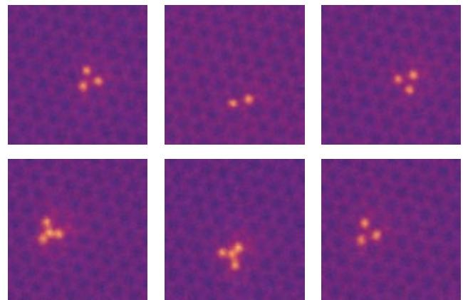
**FIGURE 3. ATOMIC MANIPULATION** can be achieved using an electron beam. Here, a cluster of silicon atoms in a graphene sheet is created and modified. (Adapted from ref. 18.)
