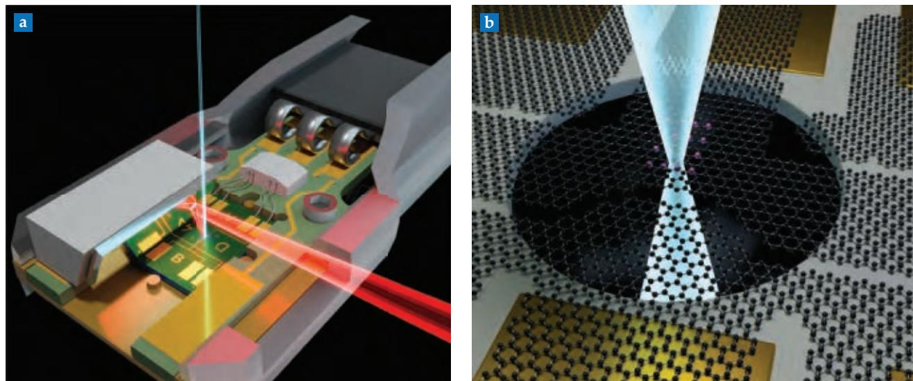
**FIGURE 4. A LAB IN A BEAM** incorporates many capabilities into one device. (a) At the microscale, lasers can heat, sculpt, analyze, or excite materials. (b) At the atomic scale, single atoms can be inserted and manipulated with an electron beam. Electrodes can be used to gate, control, or measure nanodevices.
