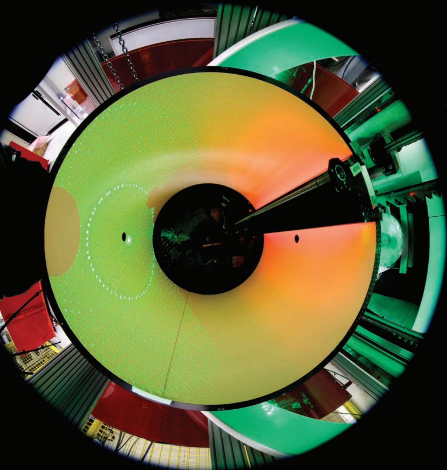
A cylindrical detector in the LADI instrument at the Institut Laue-Langevin in Grenoble, France, records neutron diffraction patterns. The data enable the generation of three-dimensional molecular structures that include hydrogen atoms. (Bob Cubitt/ILL.)
