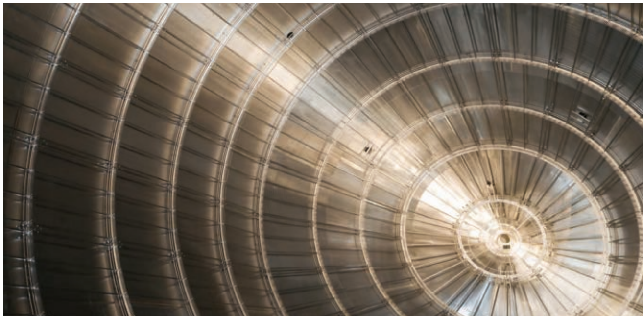
FIGURE 1. TO SEEK OUT SIGNS of neutrino masses, the KATRIN (Karlsruhe Tritium Neutrino) experiment collects and analyzes the electrons emitted in the beta decay of tritium. Successfully wrangling the electrons requires a spectrometer, the inside of which is shown here, that's the size of a house, the shape of a blimp, and permeated with a magnetic field. (Photo courtesy of M. Zacher/KATRIN Collaboration.)
