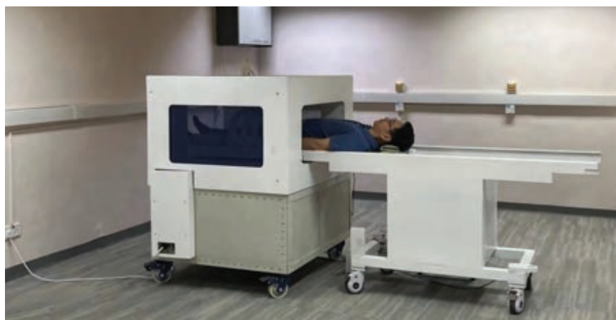
FIGURE 1. THIS MRI SCANNER operates at 0.05 T and costs much less than a conventional 3 T instrument. It can be placed in rooms that don't have expensive shielding, and its open design provides some level of comfort for patients. (Adapted from ref. 2.)
