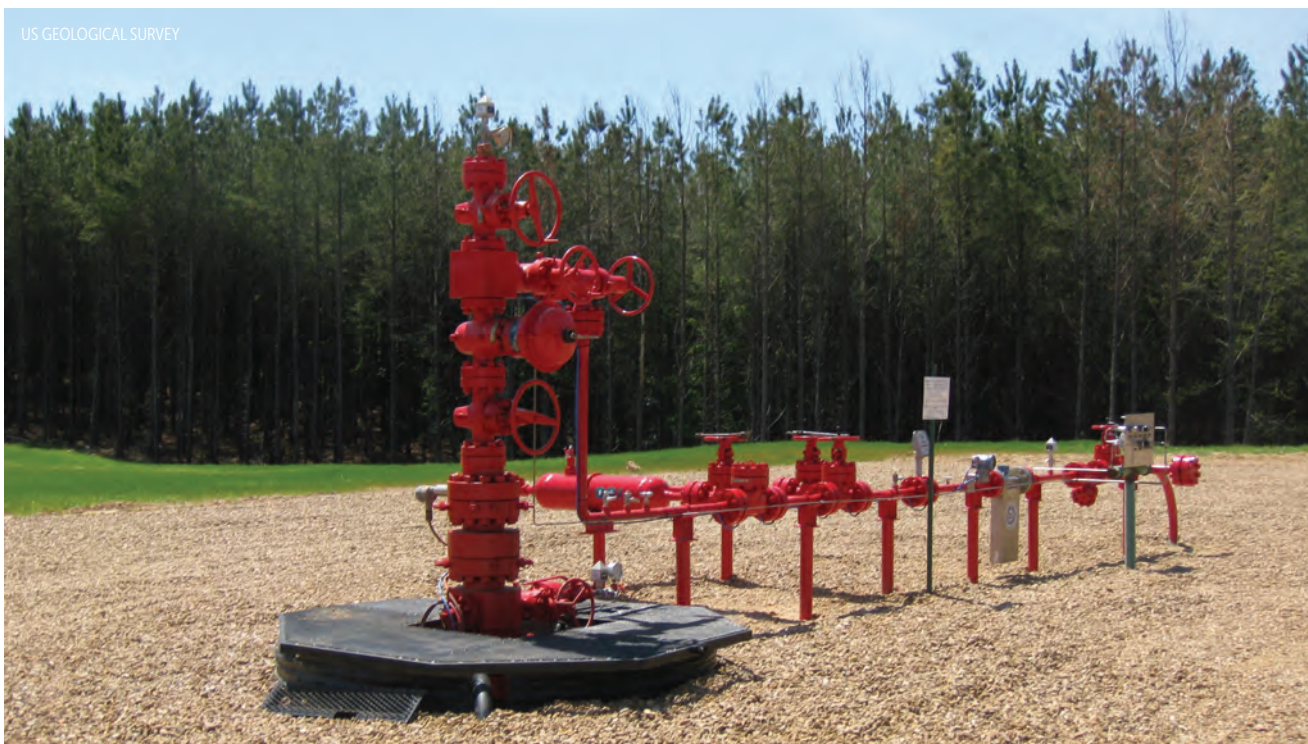
AN INJECTION WELL in Mississippi was sponsored by the Department of Energy to test the effectiveness of injecting and storing carbon dioxide in a deep saline reservoir.
