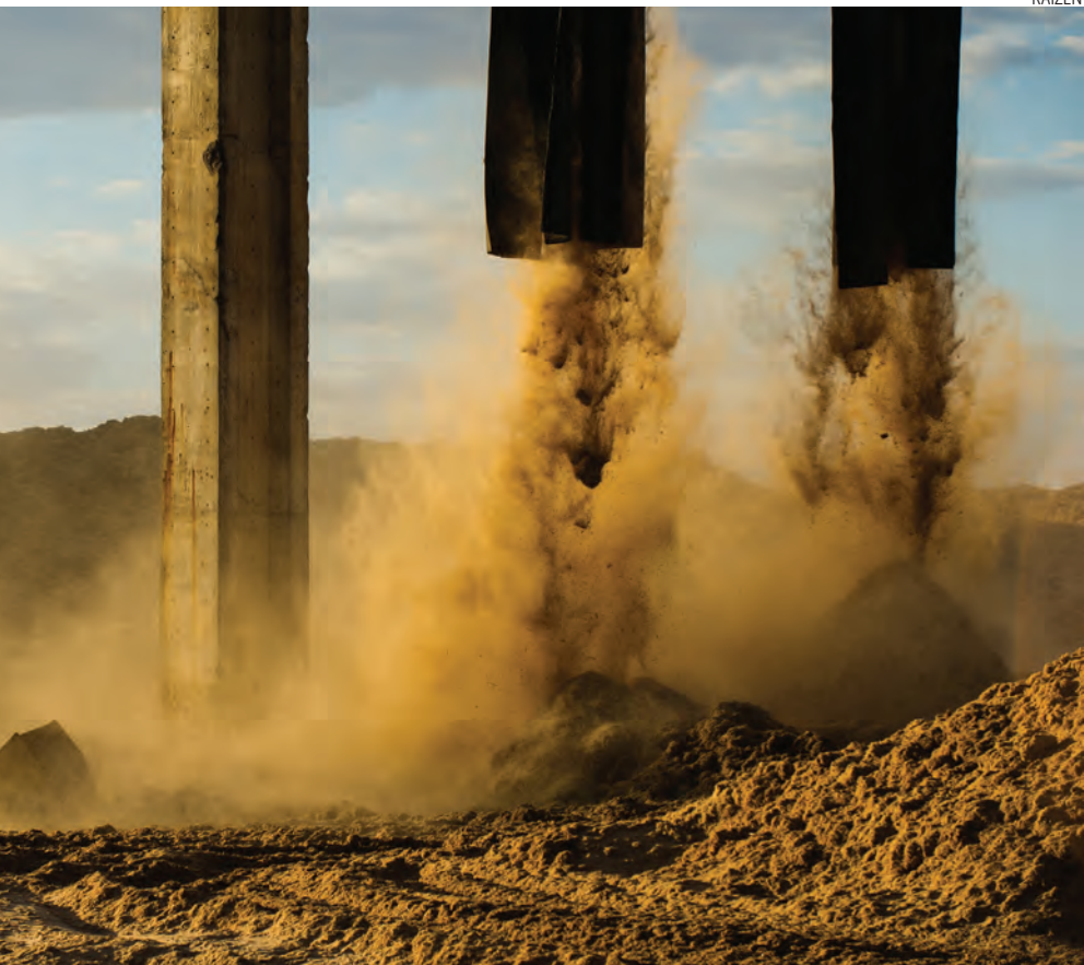
RAÍZEN'S PLANT in Piracicaba, Brazil, is the world's only commercial producer of cellulosic ethanol. Here, crushed sugarcane residue called bagasse is being loaded into the processing plant. Raízen plans to build 20 such plants by 2030.
