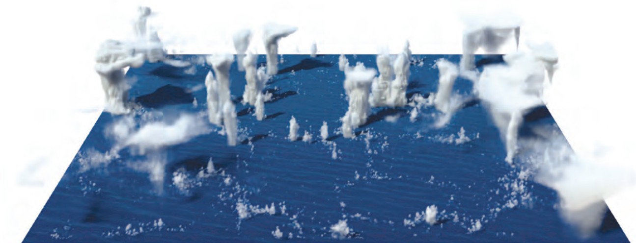
FIGURE 4. NUMERICAL MODELS are crucial for conducting climate research and estimating irreversible processes in the atmosphere and oceans. This image is a snapshot of clouds from an idealized high-resolution simulation made with the System for Atmospheric Modeling. 14 The simulation spans a 100 \times 100 \text{ km}^2 region of ocean using a horizontal grid size of 250 m. It captures many details of cloud morphology, including the tiny boundary-layer clouds that form a ring in the foreground of the image and the wispy cirrus clouds in the extreme bottom right. Processes that produce entropy irreversibly—such as mixing, evaporation, and the falling of raindrops—are not resolved and must be estimated through submodels called parameterizations.
