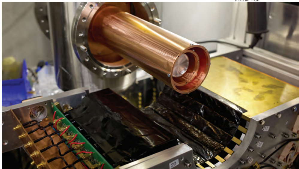
FIGURE 1. PION PHYSICS IN A TUBE. In this disassembled experiment, a 4.2-cm-diameter aluminum cylinder, just visible inside the copper radiation shields, is a vessel for holding superfluid helium. When a pion beam streams through the cylinder, some of the pions displace atomic electrons to create pionic helium atoms. A suitably tuned laser beam passing through the cylinder in the opposite direction excites some of the pionic atoms into short-lived states in which the pion and nucleus promptly and destructively collide. The fission products of the annihilated atoms, detected with an array of plastic scintillators surrounding the cylinder (half of them shown here), indicate that the laser was on resonance with an atomic transition.
