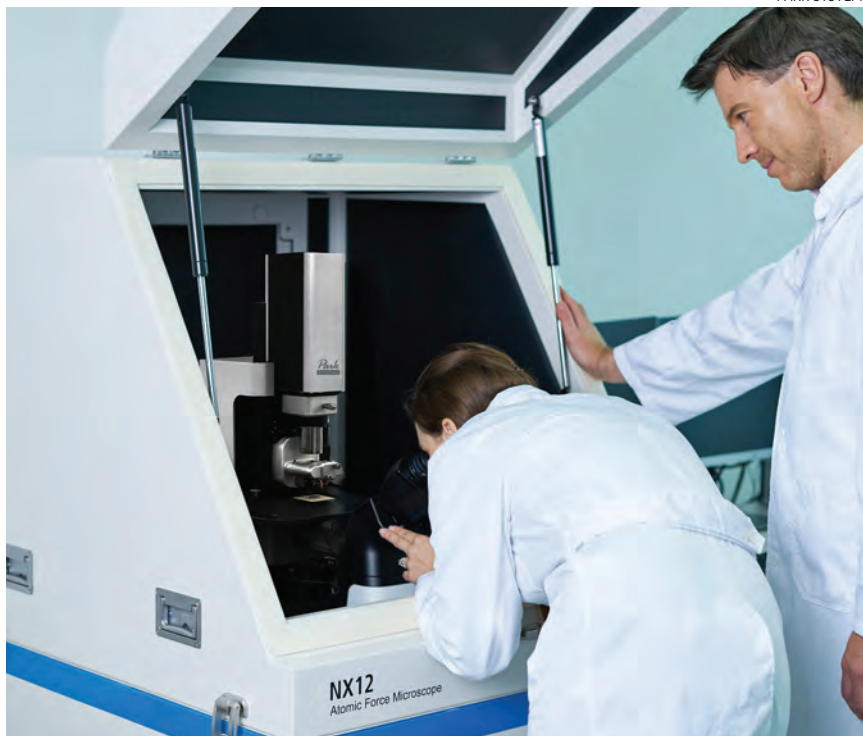
ATOMIC FORCE MICROSCOPES such as this NX12 model from Park Systems have been used for research on previous coronaviruses, including the virus that caused the severe acute respiratory syndrome pandemic in 2002.
