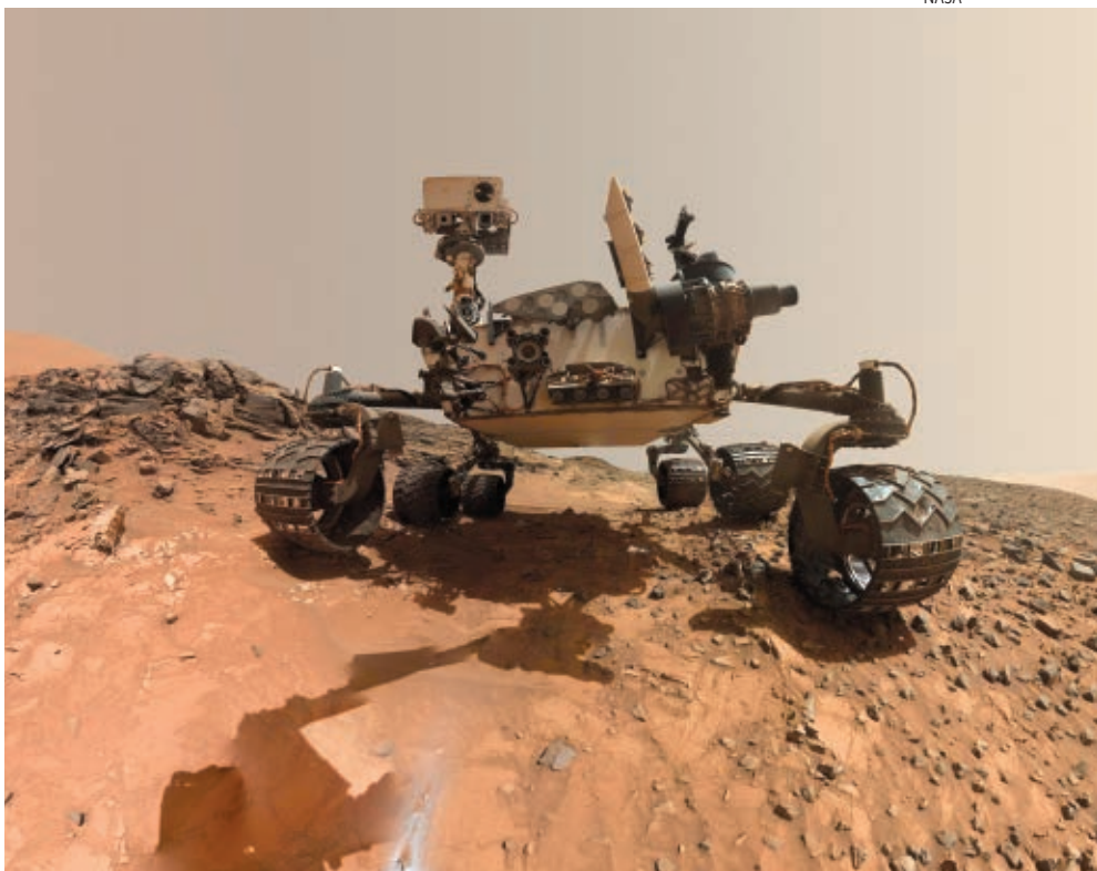
THIS SELF-PORTRAIT OF THE MARS CURIOSITY ROVER at a location known as Mount Sharp shows the dusty and rocky terrain that future astronauts may encounter. For scale, the rover’s wheels are 50 centimeters in diameter and about 40 centimeters wide.
