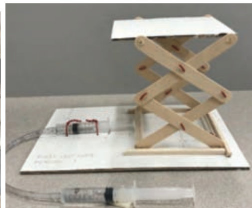
IN A PRE-ENGINEERING CLASS for which the author was the substitute teacher, a student uses a drill (left) to create the holes for bearings in a hydraulic scissor jack (right). The students used the jack to lift a cup of liquid without any spilling out.
