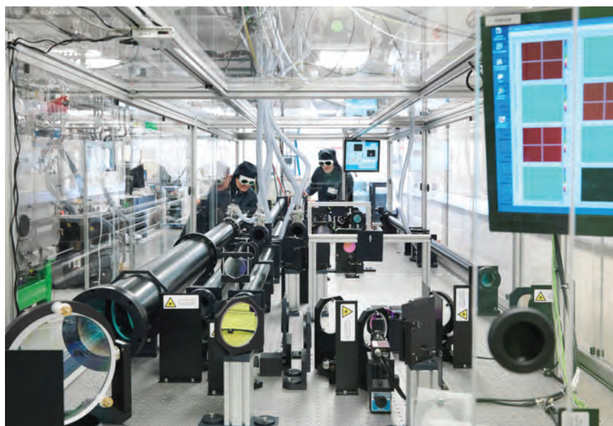
FIGURE 1. THE GEMINI LASER at the Central Laser Facility, part of the UK's Rutherford Appleton Laboratory, provided pulses for a recent experiment on laser-driven ion acceleration. Here researchers check the alignment before they send the laser beam to the target chamber. The shape of the pulses' temporal profiles resulted in the preferential acceleration of carbon ions over proton contaminants that usually dominate ion beams. The short, high-flux burst of carbon ions could be useful for research into more efficient radiotherapy treatments. (Courtesy of the Central Laser Facility, STFC.)
