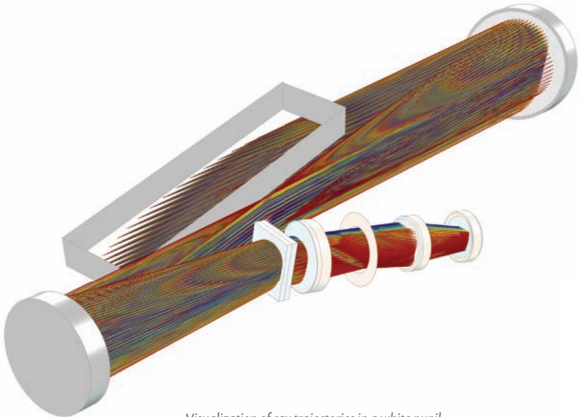
Visualization of ray trajectories in a white pupil échelle spectrograph.
