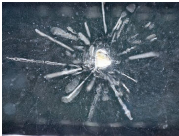
FIGURE 4. A DIFFUSION CLOUD CHAMBER , at left, homebuilt by Andrew J. C. Chong, a Malaysian physicist. At right is a close-up of the object in the chamber: a small piece of the mineral thorianite. Under the influence of the chamber's magnetic field, the thorianite emits alpha particles (thick, straight, short lines) and beta particles (thin, curvy, faint lines). (Courtesy of Andrew J. C. Chong.)
