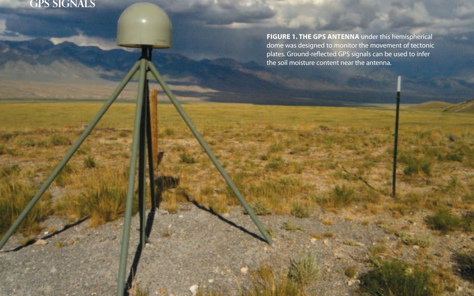
**FIGURE 1. THE GPS ANTENNA** under this hemispherical dome was designed to monitor the movement of tectonic plates. Ground-reflected GPS signals can be used to infer the soil moisture content near the antenna.
