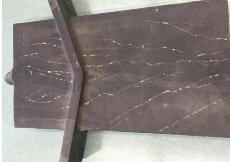
**FIGURE 1. A TURBINE BLADE** can be weakened by defects like those in this test cast. The growth direction of the freckle defects shown here is right to left, which was against gravity during the growth process. (Courtesy of Boyd Mueller of Howmet Aerospace and William Boettinger of NIST.)
