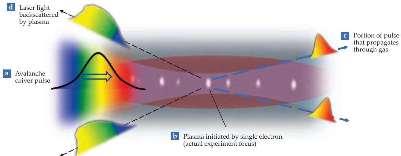
**A LASER EMITS** a short chirped pulse through air. (a) The red part of its spectrum precedes the blue. (b) Light at the laser's focus produces a plasma blob initiated by a single electron. The series of blobs pictured are experimental data. (c) Beyond the focus, a portion of the driver pulse—the early (red) part of the spectrum—continues propagating. (d) Another portion of the pulse is backscattered by the plasma. That spectrum is the main diagnostic and is collected by a spectrometer.
