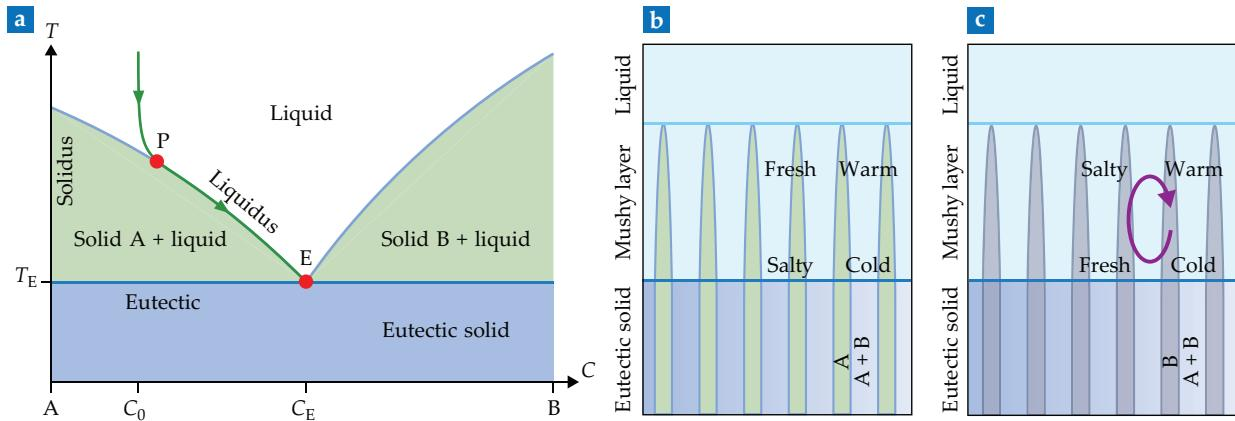
**FIGURE 2. A BINARY EUTECTIC ALLOY** with components A and B can be understood using a two-dimensional phase diagram. (a) A solution with initial composition  $C_0$  lower than the eutectic composition  $C_E$  follows path P-E along the liquidus as it gradually cools. (b) If  $C_0 < C_E$ , the residual liquid is denser than the initial melt and the mushy layer is stable. (c) If  $C_0 > C_E$ , the residual liquid is lighter, which drives convection in the mushy layer.
