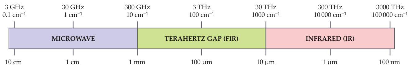
**FIGURE 1.** A GAP in the collection of molecular spectroscopic data has long existed between the microwave and IR wavelength ranges of the electromagnetic spectrum. Now technological advances are equipping far-IR (FIR) astronomers with the instrumentation they need to fill the terahertz gap.
