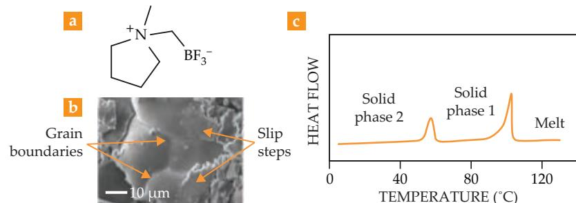
**FIGURE 2. MOST ZWITTERIONS** form crystalline phases that are unsuitable for solid-state battery electrolytes. But one newly synthesized zwitterion (a) exhibits a promising degree of disorder and plasticity. (b) An electron micrograph of the material shows small grains rife with defects. (c) A differential scanning calorimetry trace reveals a solid–solid phase transition, a known sign of an organic ionic plastic crystal. (Adapted from ref. 1.)
