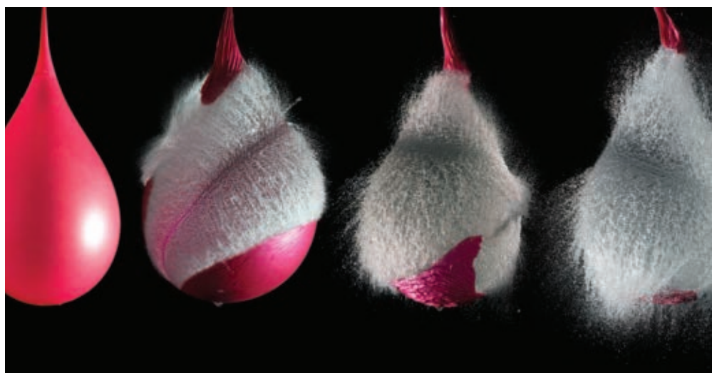
FIGURE 1. IN THE BLINK OF AN EYE , a single pinprick can prompt an inflated balloon (shown here filled with water) to tear itself to shreds: The energy stored in the stretched latex is more than enough to power the rapidly propagating cracks. When less energy is available, damage in an elastic solid develops more slowly. The molecular details of material failure are key to how the process plays out. (Image by Jose Luis Stephens/Shutterstock.com.)
