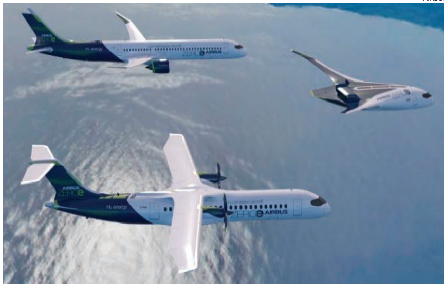
THREE CONCEPTUAL HYDROGEN-FUELED airliners from Airbus all combine hydrogen-burning gas turbines with hydrogen fuel cells that generate electrical power. The turboprop (bottom) would carry up to 100 passengers and have a range of 1000 nautical miles. The others would carry up to 200 passengers, with a range of 2000 nautical miles.
