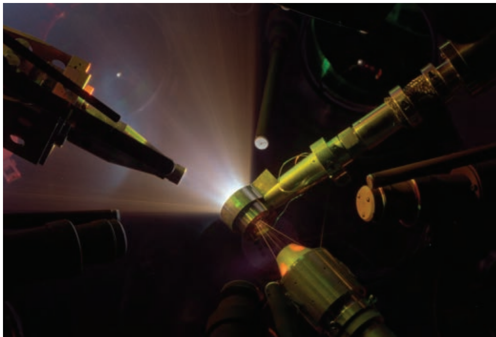
FIGURE 1. COMPRESSION EXPERIMENTS. At the University of Rochester's Laboratory for Laser Energetics, researchers uncovered new phase behavior in a mixture of hydrogen and helium gas. The cylindrical diamond anvil cell in the center of the photo compressed the gas sample statically before a laser-induced shock wave propagated through the sample and squeezed it dynamically to the pressure and temperature range of Jupiter's interior. (Photo courtesy of OMEGA Laser Facility.)
