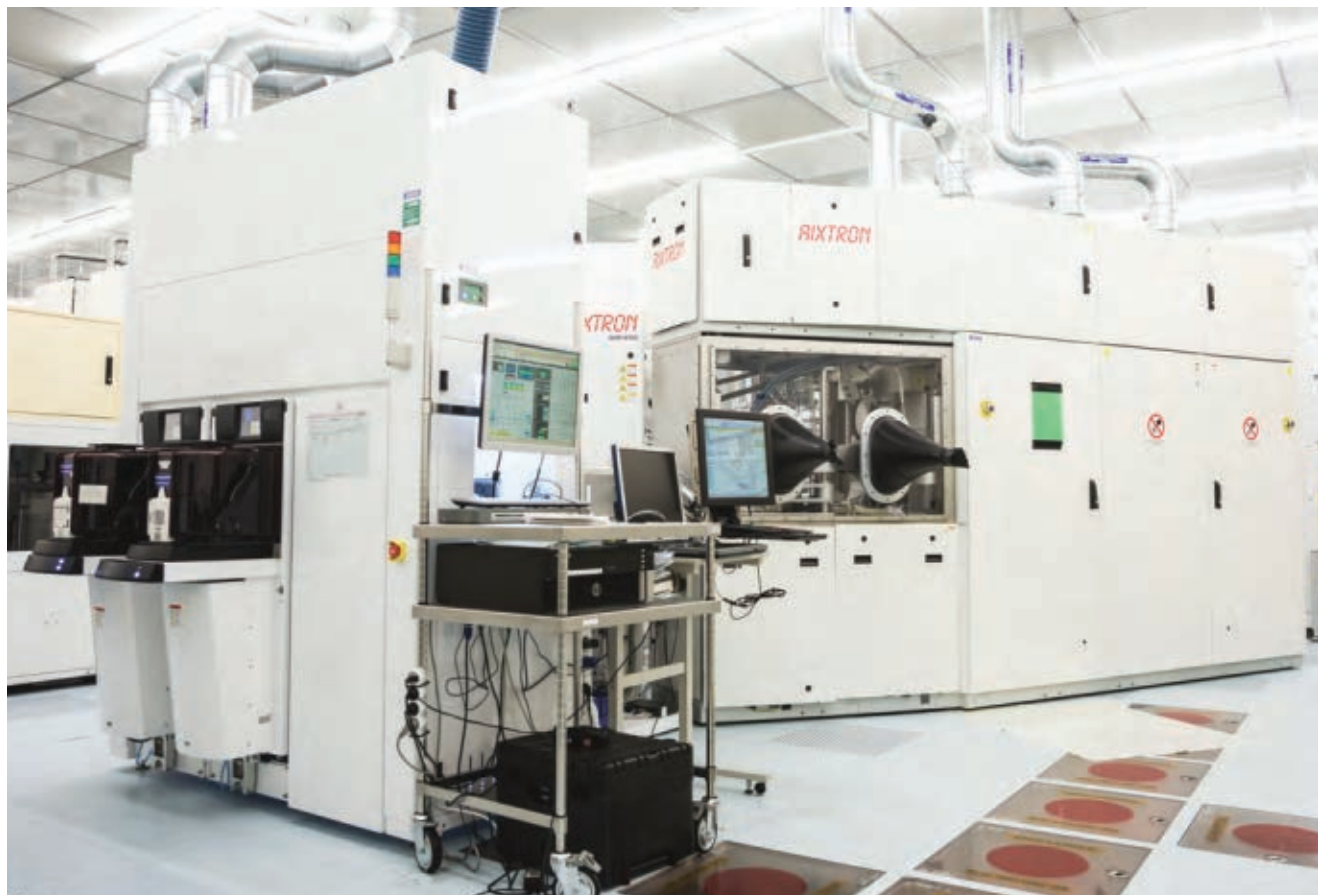
AIXTRON MACHINES perform chemical vapor deposition of graphene for compound semiconductor applications. The technology was developed by the German company through the Graphene Flagship.
