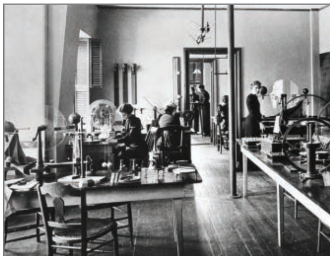
FIGURE 2. A ROOM IN WELLESLEY'S PHYSICS LABORATORY, CIRCA 1893. The instrumentation includes various electrostatic generators, or Wimshurst machines, Leyden jars, induction coils, and a galvanometer. It was only the second undergraduate physics laboratory in the country, and the first for female students. (Courtesy of Wellesley College Archives, Library & Technology Services.)
