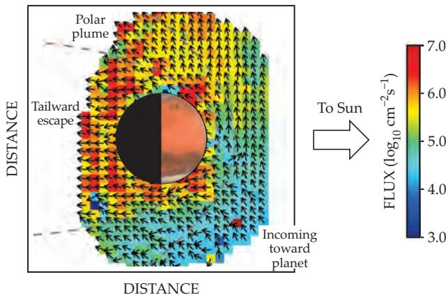
**FIGURE 2. A YEAR'S WORTH** of data on oxygen escaping from Mars. Colors represent the flux of oxygen atoms, and arrows show the average direction of their movement. (Adapted from an image courtesy of the American Geophysical Union.)
