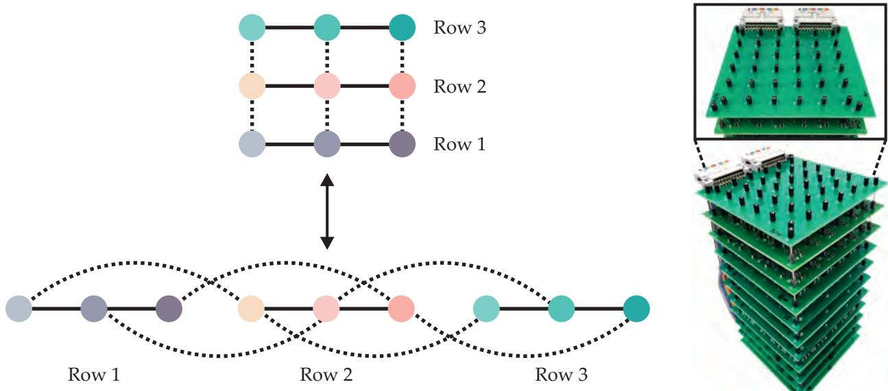
**FIGURE 2. HIGHER-DIMENSIONAL LATTICES** can be constructed in lower-dimensional systems. On the left, a two-dimensional discrete lattice model is composed of lattice sites (circles) with connections (lines). That same lattice can be effectively embedded into one dimension provided the same connectivity is maintained. On the right, that embedding trick was used to encode a 4D lattice into this 3D stack of circuit boards. (Photo from ref. 9.)
