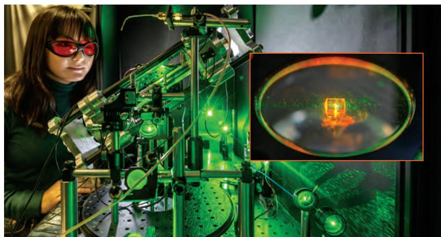
**FIGURE 1. NO VACUUM CHAMBERS** are needed to study surface chemistry using diamond NV-center NMR. Here, Kristina Liu of the Technical University of Munich operates the relatively simple experiment, which uses green light from an inexpensive solid-state laser to read the NV centers' spin states. The 2-mm-square diamond, not visible in the main image, is shown in the inset. (Photos by Andreas Heddergott, Technical University of Munich.)
