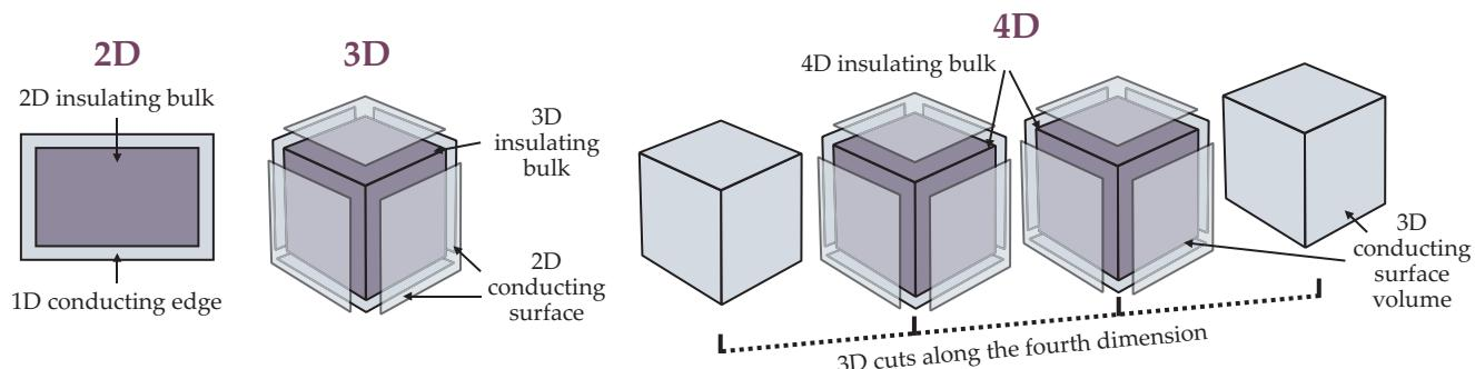
**FIGURE 1. TOPOLOGICAL INSULATORS** in two, three, and four dimensions conduct on their edges or surfaces (light gray) despite an insulating bulk (violet). That unusual behavior results from the topology of the electronic band structure. In 3D and 4D systems, the conducting surfaces are depicted lifted off the bulk to show it and the surface simultaneously. The 4D topological insulator is shown as several separate 3D cuts along the fourth dimension.
