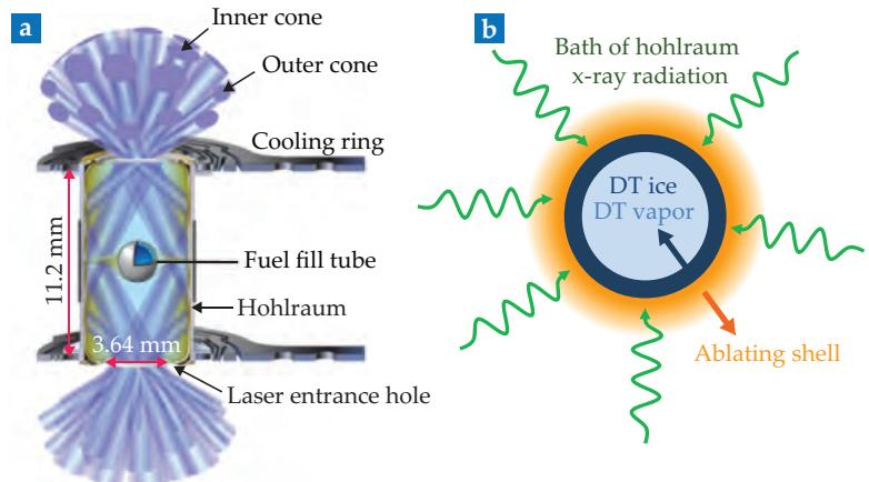
**FIGURE 2. INERTIAL CONFINEMENT FUSION** uses indirect laser excitation to spark a burning plasma. (a) Laser beams enter the hohlraum at various angles through top and bottom holes and heat its interior wall. (b) The flux of soft x rays reradiated by that wall expels the capsule's outer shell. By conservation of momentum, its inner shell of frozen and gaseous deuterium and tritium (DT) fuel is driven inward. (Adapted from ref. 1.)
