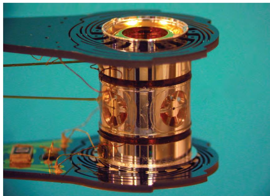
**FIGURE 1. A GOLD CYLINDER** known as a hohlraum holds a fuel capsule at its center for fusion experiments at the National Ignition Facility. Target-handling systems precisely position the capsule and cool it to cryogenic temperatures. (Courtesy of Lawrence Livermore National Laboratory.)
