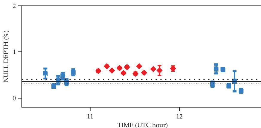
**FIGURE 3. THE NULL DEPTH** embodies the amount of circumstellar emission detected through nulling interferometry. The offset between the data for Vega (red), a star from the Hunt for Observable Signatures of Terrestrial Planetary Systems survey, and those for calibration stars (blue) indicates a glow from exozodiacal dust in Vega's habitable zone. The dotted lines represent the one-sigma uncertainty of the null floor.
