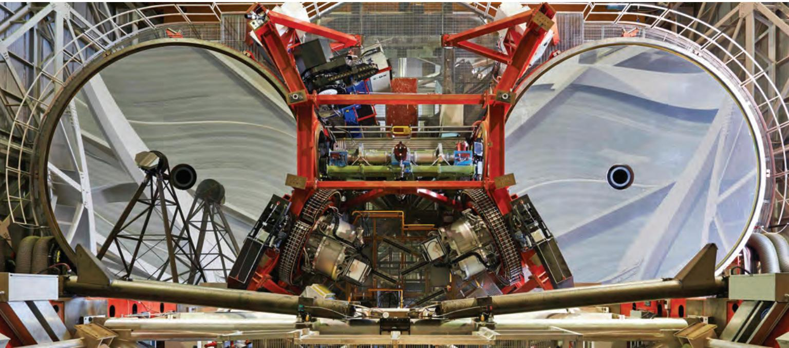
**FIGURE 2. THE TWIN APERTURES** of the Large Binocular Telescope sit 14.4 m apart, center to center. The green structure between them is an interferometer that enables the telescope to be used for nulling. (Courtesy of LBTO—Enrico Sacchetti.)
