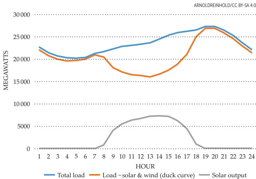
**THE DUCK CURVE** is the daily load pattern from natural gas power plants and other on-demand sources of electricity that occurs in states with large amounts of distributed solar energy. Electric vehicle charging in the evening will exacerbate the peak demand that already occurs after the Sun sets. These data are from California on 22 October 2016.
