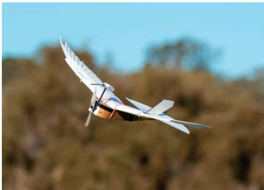
FIGURE 1. THIS BIOHYBRID ROBOT combines mechanical parts with pigeon feathers. During real-world flight tests with high and low turbulence, PigeonBot controlled the position of its 40 feathers using four wing-mounted motors. The feathers’ fasteners prevented any gaps in the wings from forming that would have otherwise limited the robot’s mobility. (Lentink Lab/Stanford University.)
