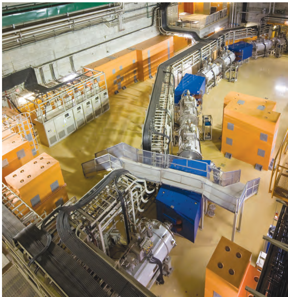
FIGURE 1. THE RADIOACTIVE ISOTOPE projectile separator BigRIPS enabled researchers to isolate enough magnesium-40 for gamma-ray spectroscopy. The separator was part of the upgrade to RIKEN's facility in 2007 and is used to separate the isotopes produced by the primary beam's breakup into secondary beams. BigRIPS allows for higher-intensity beams than its predecessor, RIPS, because of its larger apertures and two-stage separation scheme. (Photo courtesy of RIKEN Nishina Center.)
