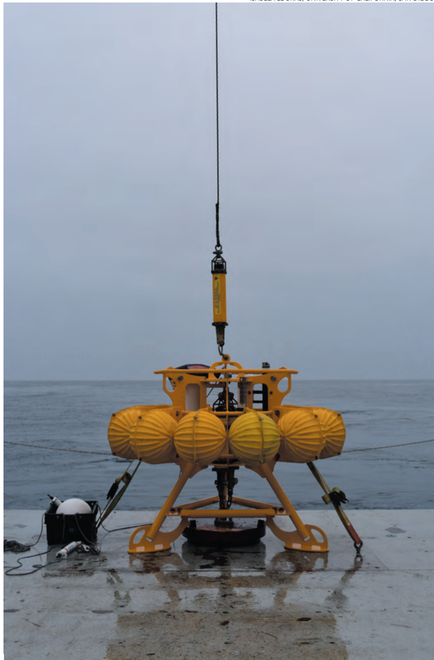
FIGURE 2. THE MOORING SHOWN HERE will sit on Greenland's continental shelf 200 m below the surface. While the yellow portion anchors the mooring to the seafloor, the instruments in the black box to the left float above it and collect continuous measurements of temperature, salinity, and velocity at multiple depths.
