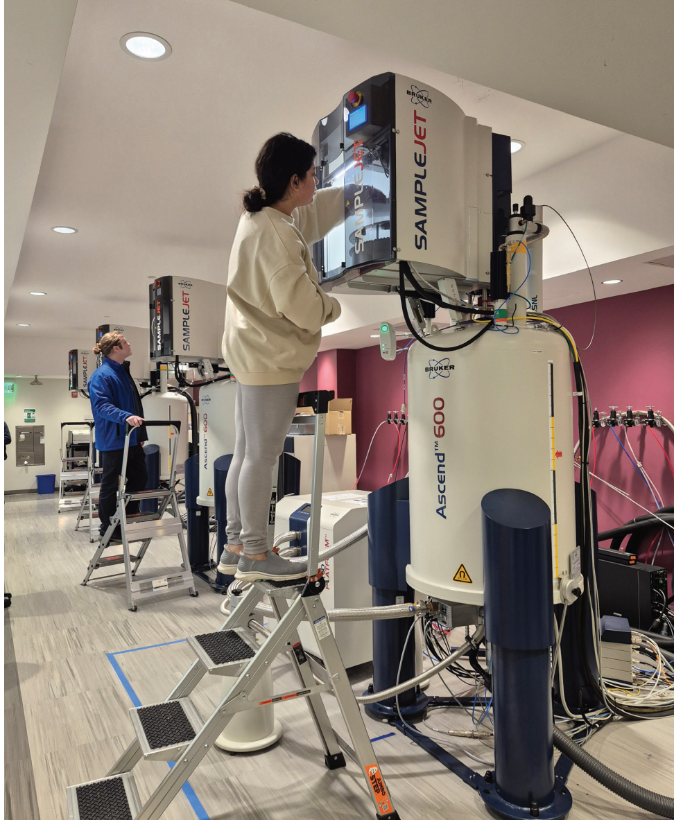
◀ Apala Chaudhuri places clinical samples into Olaris's NMR spectrometer. Any interruption in helium would translate to an interruption in patient care, CEO Liz O'Day says. (Photo courtesy of Liz O'Day.)
