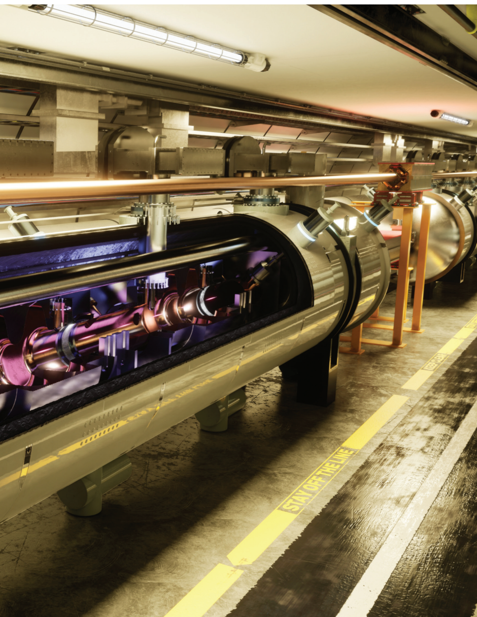
◀ An artistic representation of the Future Circular Collider. Some 102 cryomodules, several of which are shown, would contain a total of 408 RF cavities and accelerate the electrons and positrons to center-of-mass energies ranging from 88 GeV to 365 GeV. (Image created by the CERN audiovisual team, courtesy of CERN.)
