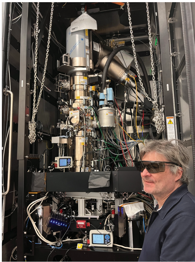
▲ Figure 3. Holger Müller in front of the laser phase plate–fitted electron microscope. (Photo courtesy of Robert Sanders/UC Berkeley.)
