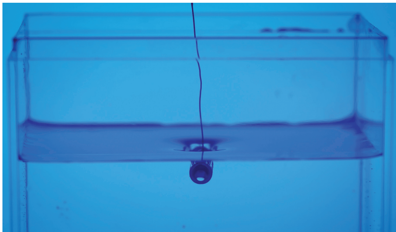
▲ Figure 1. An aluminum tube displaces water around it as it is lowered into the water. Once water covers the top of the tube, a trapped air bubble allows the tube to maintain the required buoyancy to stay afloat. (Photo courtesy of the University of Rochester.)
