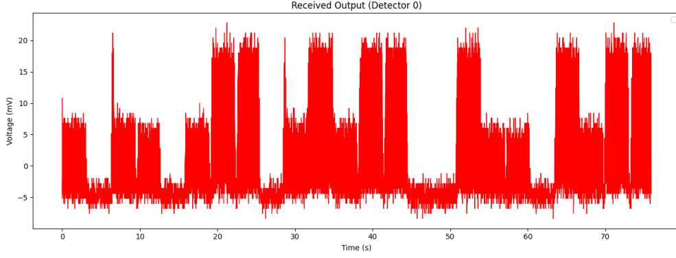
(a) Oscilloscope reading for detector 0. A high voltage output corresponds to a received 0 bit, and a low voltage corresponds to a received 1 bit. Middle-level voltages correspond to mismatched bases.
