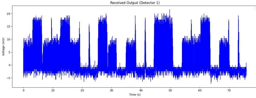
(b) Oscilloscope reading for detector 1. Conversely, a high voltage corresponds to a received 1 bit, while a low voltage corresponds to a received 0 bit.
