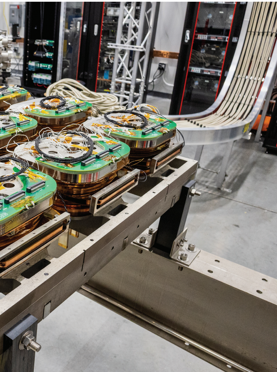
◀ High-temperature superconducting planar coils are being used by Thea Energy to simplify its stellarator design. The company has tested the coils; the next step is to build a prototype stellarator, which is scheduled to be operational by 2030. (Photo courtesy of Thea Energy Inc.)
