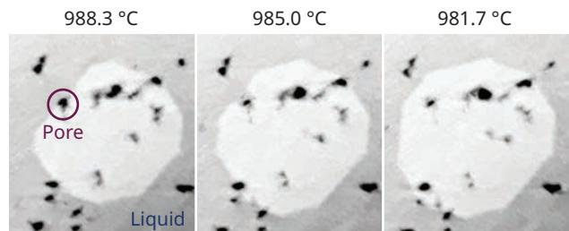
▲ Figure 1. A quasicrystal grows defect-free. As a 150-μm-wide, 10-sided quasicrystal (white) cools and solidifies from an aluminum-cobalt-nickel liquid alloy over a few minutes, it encounters shrinkage pores (black specks). The obstacles initially distort the shape of the quasicrystal. But because of its ability to rearrange its lattice points while preserving the ordered structure, the quasicrystal forms without defects. (Images courtesy of Insung Han and Ashwin Shahani.)
