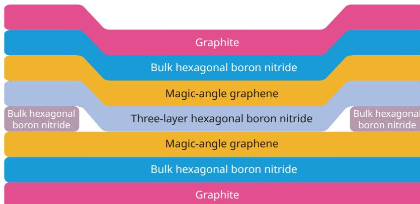
▲ Magic-angle graphene superconducts at low temperatures, but probing the energetics of the superconducting state has been a challenge. With this multilayered device, researchers can simultaneously measure the charge transport and density of states of the elusive superconductor. (Figure adapted from ref. 1 by Freddie Pagani.)
