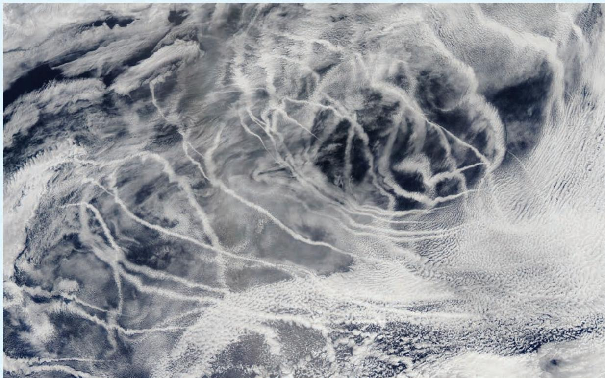
▲ **Figure 3.** Aerosol emissions from ships can seed cloud formation and create ship tracks—a similar effect to marine cloud brightening aimed at increasing the reflection of solar radiation. (Image courtesy of NASA Goddard Photo and Video photostream, NASA/GSFC/Jeff Schmaltz/MODIS Land Rapid Response Team.)
