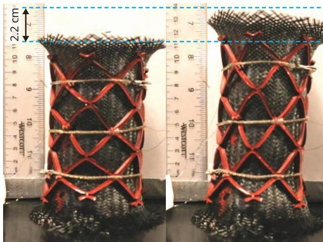
◀ **Figure 2.** When an octopus-inspired sleeve is squeezed, it elongates by almost 20%. The motion is initiated by three twisted and coiled artificial muscles (brown) that are wrapped horizontally around the soft structure. In response to external stimuli, such as heat, the muscles contract and squeeze the composite sleeve. The red elastomer mesh distributes the load over the sleeve. (Image adapted from P. Kotak et al., *Soft Robot.* **11**, 432, 2024.)
