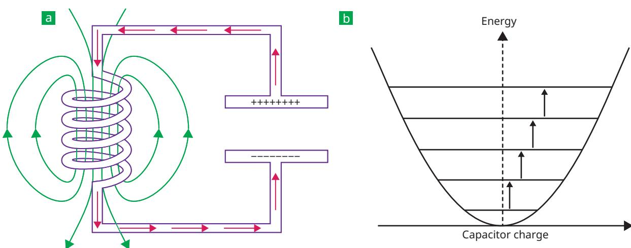
▲ **Figure 1.** In an inductor–capacitor circuit (a), charge bounces between the plates of the capacitor like a mass on a spring. The harmonic-oscillator potential (b) gives rise to a series of discrete energy levels. But because the levels are all equally spaced, observing their quantization would be difficult. (Figure by Freddie Pagani.)
